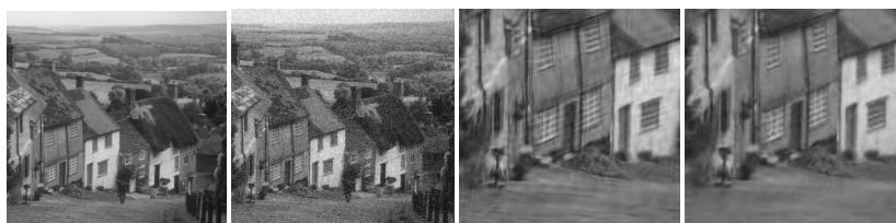
FIGURE 1. Denoising of the Goldhill image ( 512 \times 512 ) using shearlets and curvelets. Left to Right : Original image, Noisy image (PSNR 20.17 dB), Curvelet-denoised image (PSNR 28.70 dB/ Computing time 7.22sec), Shearlet-denoised image (PSNR 29.20 dB / Computing time 5.56sec).
