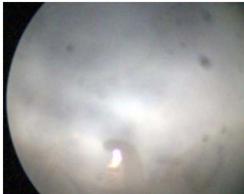
Figure 9 : Bulk auto-ignition at the same time as the spark (processed image)
