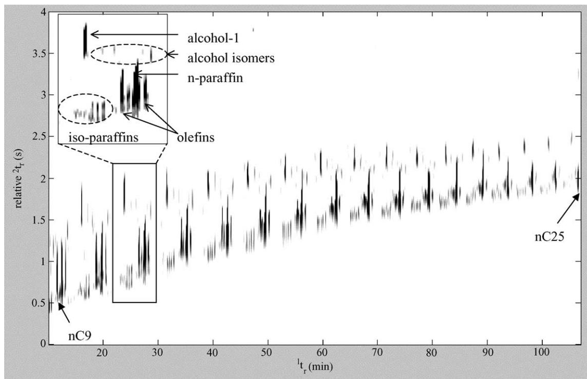
Fig. 3. GC  $\times$  GC analysis of a Fischer-Tropsch product. Experimental conditions: Table 1. The repetitive pattern representing the distribution of isoparaffins, olefins, and alcohols in the elution zone of a normal paraffin is enhanced in the upper left part of the chromatogram.
