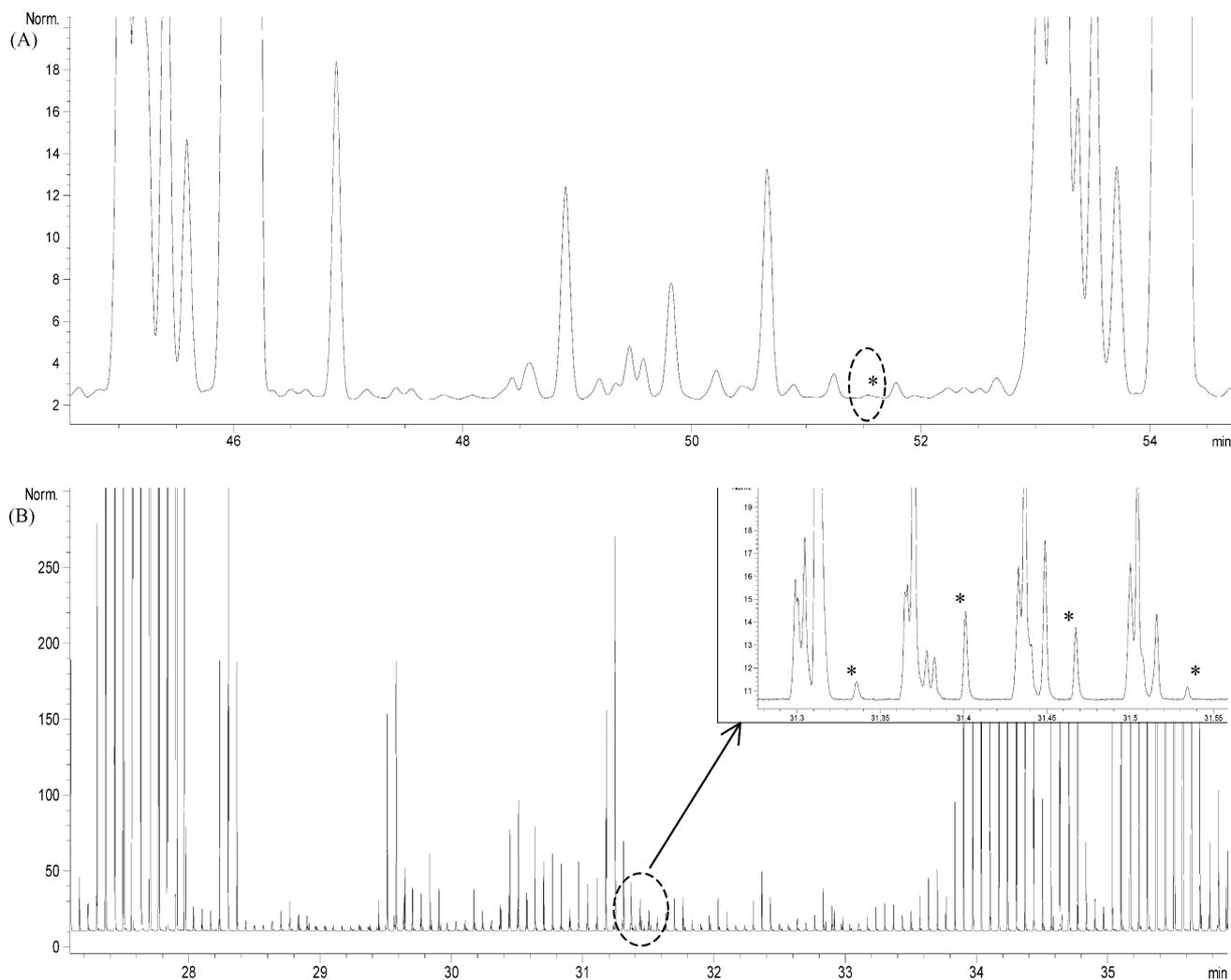
Fig. 2. Dehydrogenation of *n*-paraffins: chromatograms of the product converted at 20% obtained in 1D-GC (A) and in GC  $\times$  GC (B). The elution zone of naphthalene is circled with a dotted line and has been highlighted in the insert of (B). Naphthalene is indicated with the symbol \*. Experimental conditions: see Table 1 (B) and Table 2 (A).
