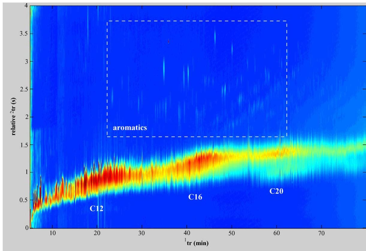
Fig. 4. GC  $\times$  GC chromatogram of a product of oligomerization. Experimental conditions: see Table 1. The elution zone of alkylbenzenes is framed with a dotted line.
