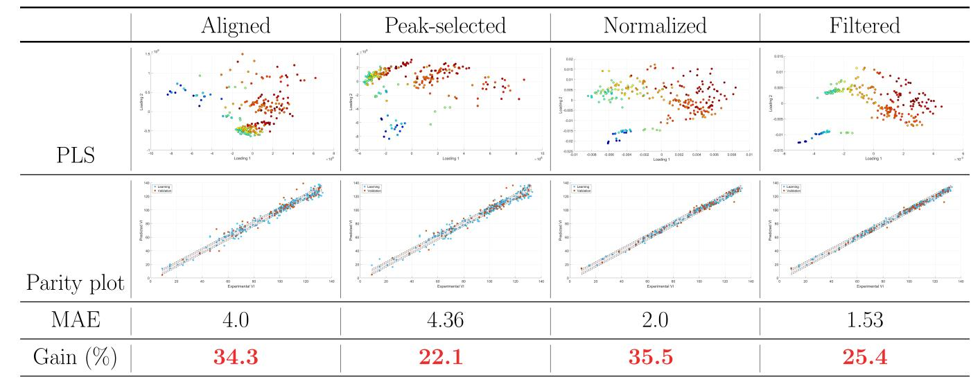
• MAE and Gain using SG filtering
