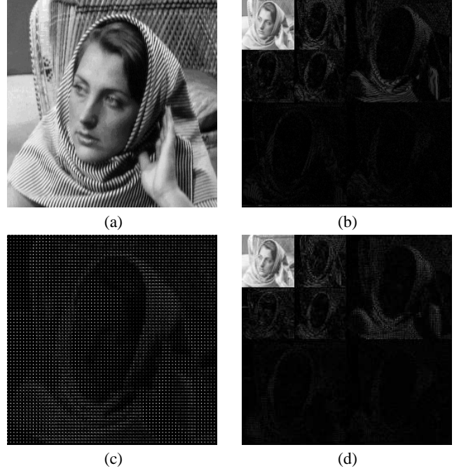
Fig. 4. (a) Original Barbara image, (b) Wavelet-db8 decomposition, (c) four-channel DCT block decomposition, (d) dyadic re-mapping from image (c).
